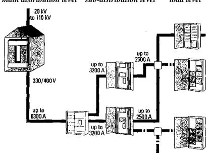
Power is thus supplied to the electrical loads via the low-voltage switching station, main distribution board, sub-distribution board and small distribution board by means of a low voltage, e.g. 230/400 V. The electrical connections between these components are established via different cables and electric lines as well as busbar trunking and installation systems.
