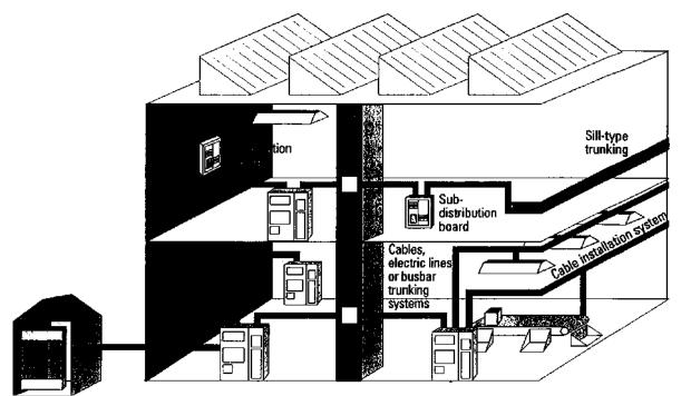
Fig. 1.1/2 shows the most important components that are required for distributing power in an industrial or functional building.
