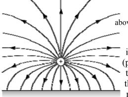
Pic.3. Field lines emanating from a positive charge above a plane conductor
